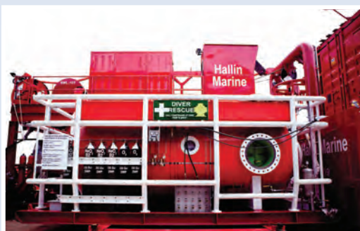
Hallin's modular saturation diving system on the Carlisle will be used to support dive teams.
