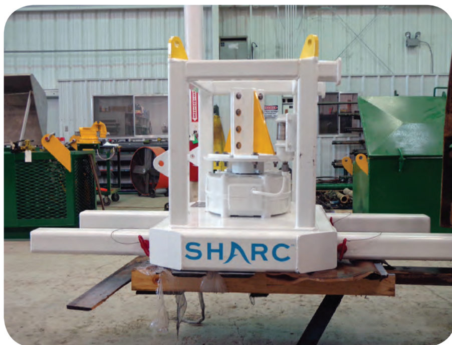
The SHARC cutting head is secured in a frame that attaches to the exposed tubular.
