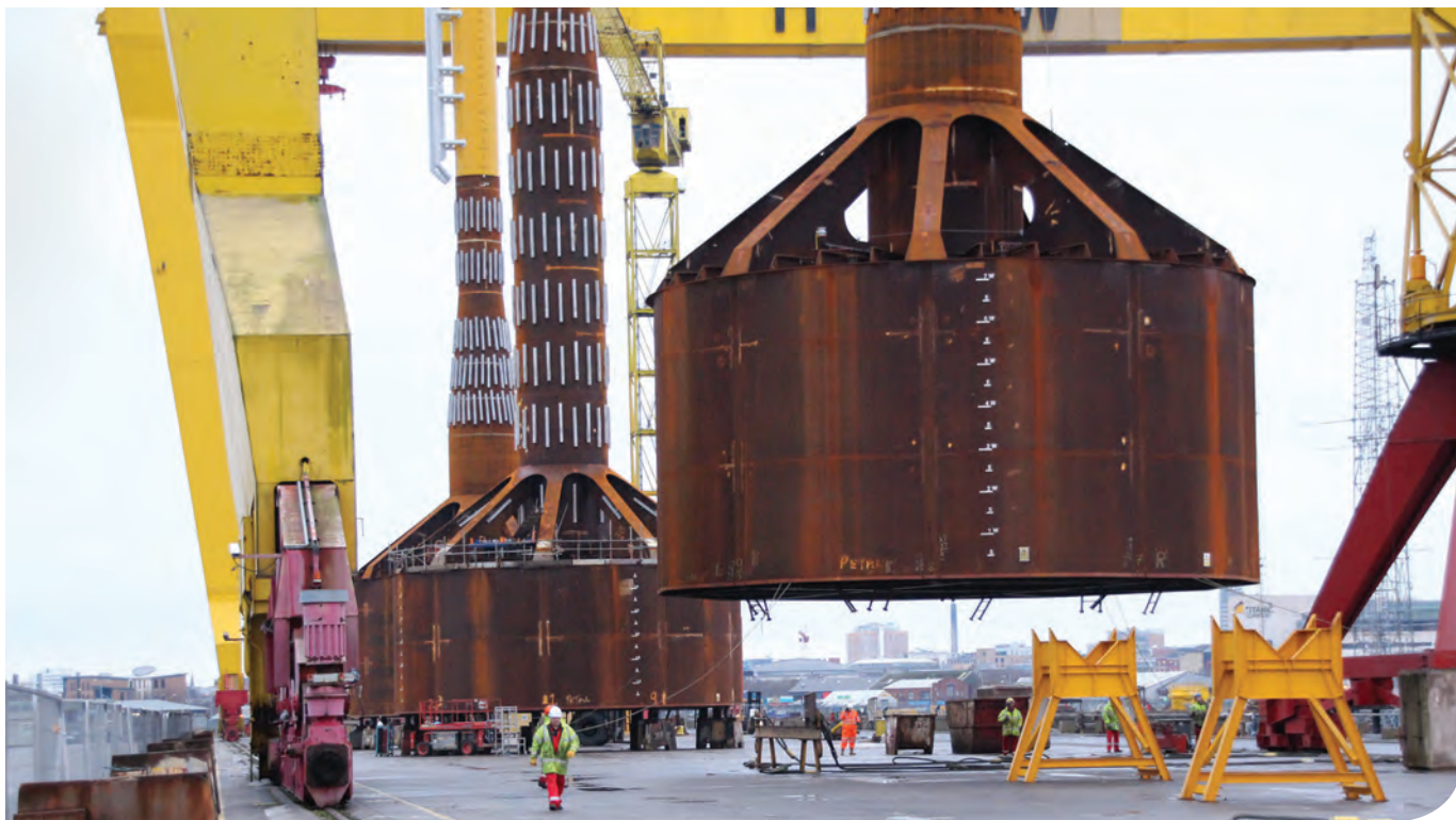
Several bucket foundations are shown during manufacture at the Harland & Wolff shipyard in Belfast, Northern Ireland. The worker walking underneath gives a perspective on the dimensions of the upturned bucket design. Photo: Fred. Olsen United
