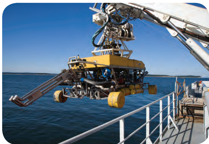
Nexans owns and operates three complete Capjet trenching machines with dedicated launch and recovery systems.
