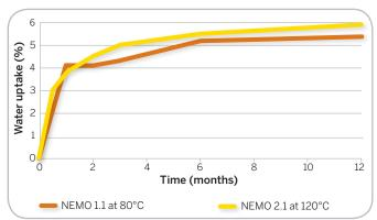
Fig. 5: Water uptake in NEMO 1.1 and 2.1 during hot-wet exposure at 80°C and 120°C, respectively.
