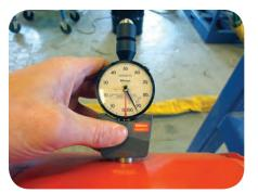
**Fig. 6:** Shore A Hardness Durometer is used to measure the hardness of the joint after demold time and after 24hr. The acceptance criterion is ≥55 at demold and 90±10 Shore A after 24hr.
