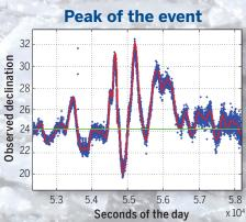
improvement of real-time declinations over modeled declinations for marine seismic streamer positioning in the Arctic.
