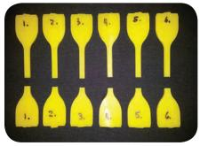
Fig. 9: Two series of six plaques measuring 150x45x13mm were machined from NEMO 2.1 material to establish the elastic modulus of the material. Tensile bar dimensions were as per ASTM D638-03 Type IV.
