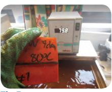
**Fig. 7:** A 100mm x 100mm test specimen of NEMO 1.1 was immersed in the water bath at 80°C for 48hr. There was no edge disbondment and passed the acceptance criteria with Rating 1.
