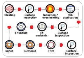
Fig. 3: The NEMO system coating application process.
