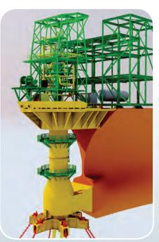
A schematic of LMC's external turret system design for the FSRU *Toscana*. Image: LMC.
