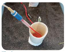
Fig. 8: A 100mm x 100mm test specimen of NEMO 1.1 was setup for a cathodic disbondment test for 28 days at 95°C in 3% NaCI solution and -1.5V. The average disbondment was 8.8mm and met the acceptance criteria of ≤20mm.
