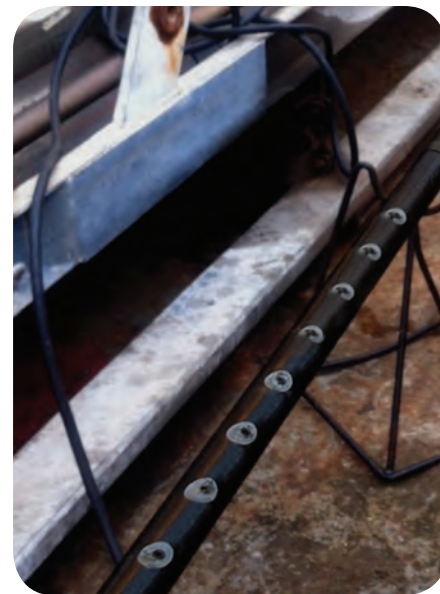
Recovery of perforating guns after use in open water. Photos: Reaching Ultra.
