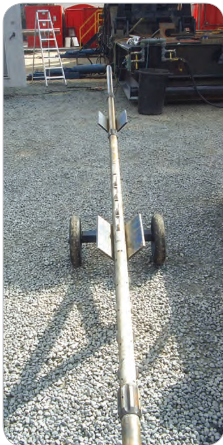
Forward/reverse wheeled sections of wireless tractor. Photo: BP.
