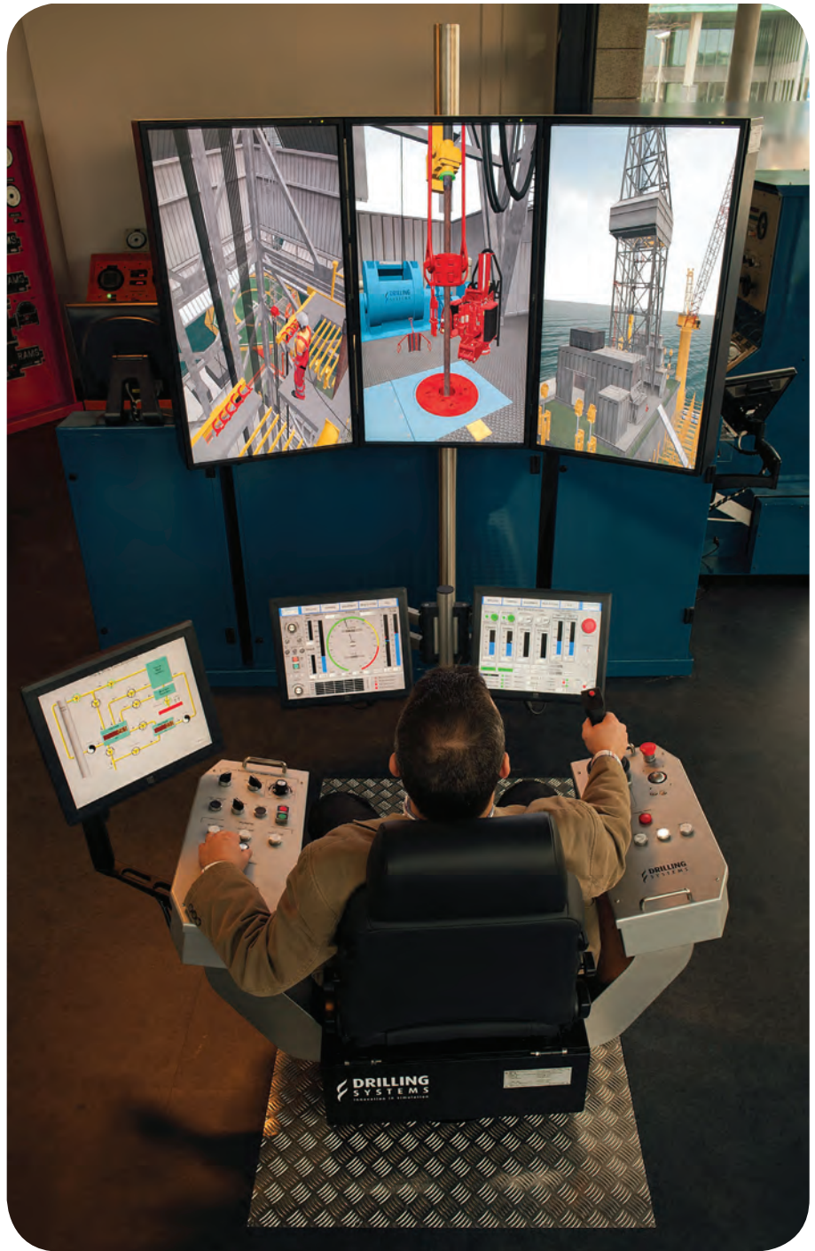
Trainees can use the DrillSim 5000 to perform drilling and well control simulations as a part of Shell's Advanced Well Control Training Program. Photo: Shell
