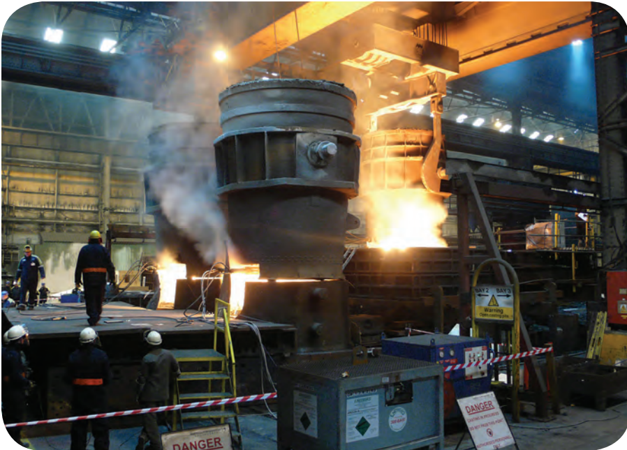
Three ladles pour the liquid steel into the mold.
