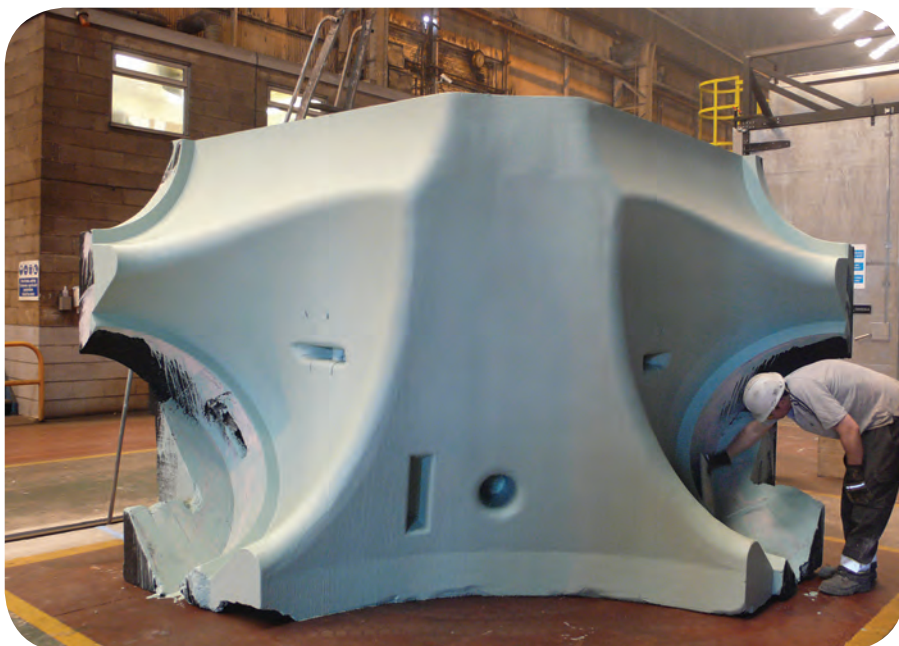
A completed mold section.
