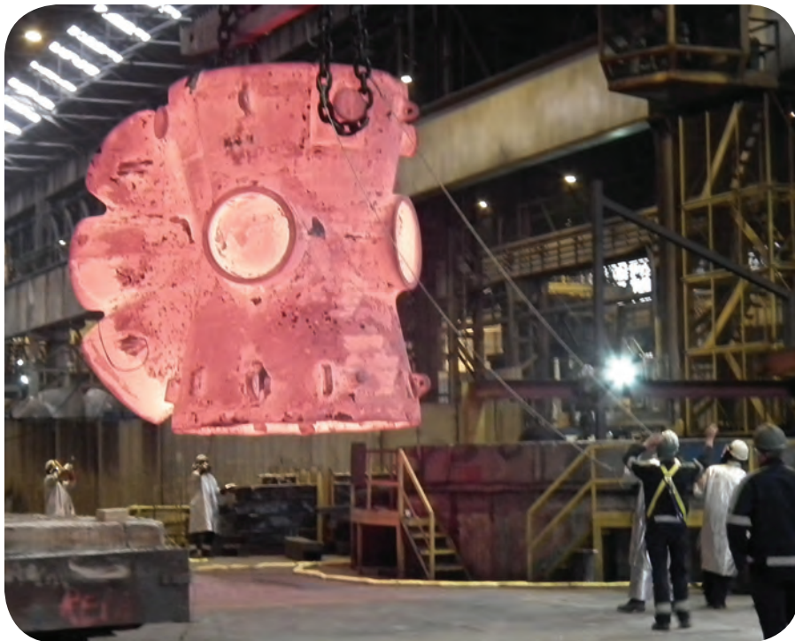
A truss node is taken from the furnace for quenching, with the quench tank in the background. Images: Vulcan SFM.
