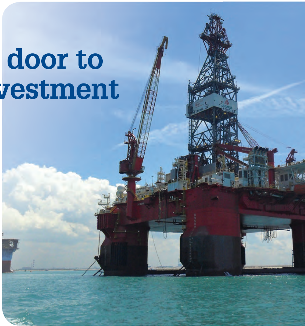
A 6th generation DP semisubmersible, Pemex's Centenario GR is capable of drilling in 3000m (10,000 ft) water depth. More than 85% of the rigs working offshore Mexico are classed by ABS. Photo courtesy of Grupo R
