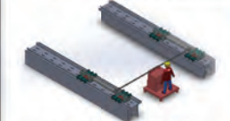
Skidding system with locking mechanism on vessels.
