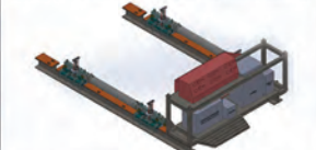
Skidding system with locking mechanism and wireless handheld controls on vessels.
