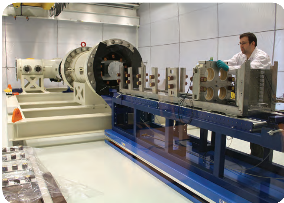
The switchgear in assembly. Photo by Elaine Maslin.
