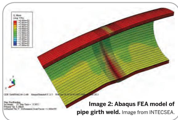
**Image 2: Abaqus FEA model of pipe girth weld.** Image from INTECSEA.
