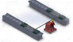
Skidding system with locking mechanism on vessels.
