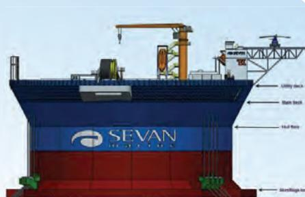
**A moonpool was added to specs for a Sevan-designed circular FPSO to accommodate steel catenary risers.** Images from Sevan Marine.
