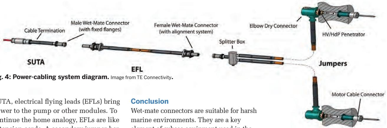
Fig. 4: Power-cabling system diagram. Image from TE Connectivity.
