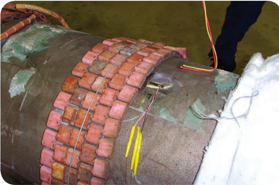
**Image 3: Temperature is an important component in pipe performance and simulation models replicating such performance require accurate data capture. Here, a pipe is wrapped in a heating blanket as it is brought up to 130°C, replicating the effect of high temperature well fluids.**
