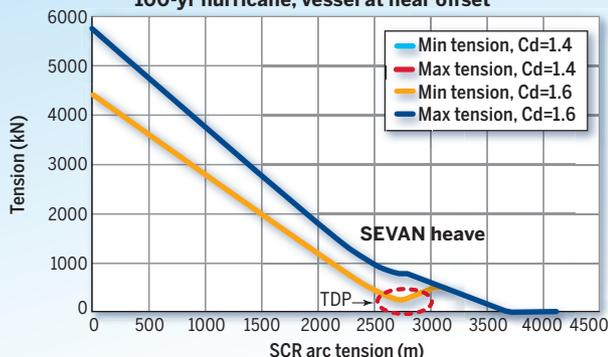
Minimum and maximum tensions along riser arc length, 100-year hurricane (Load Case No. 4). Sensitivities on  $C_d$
