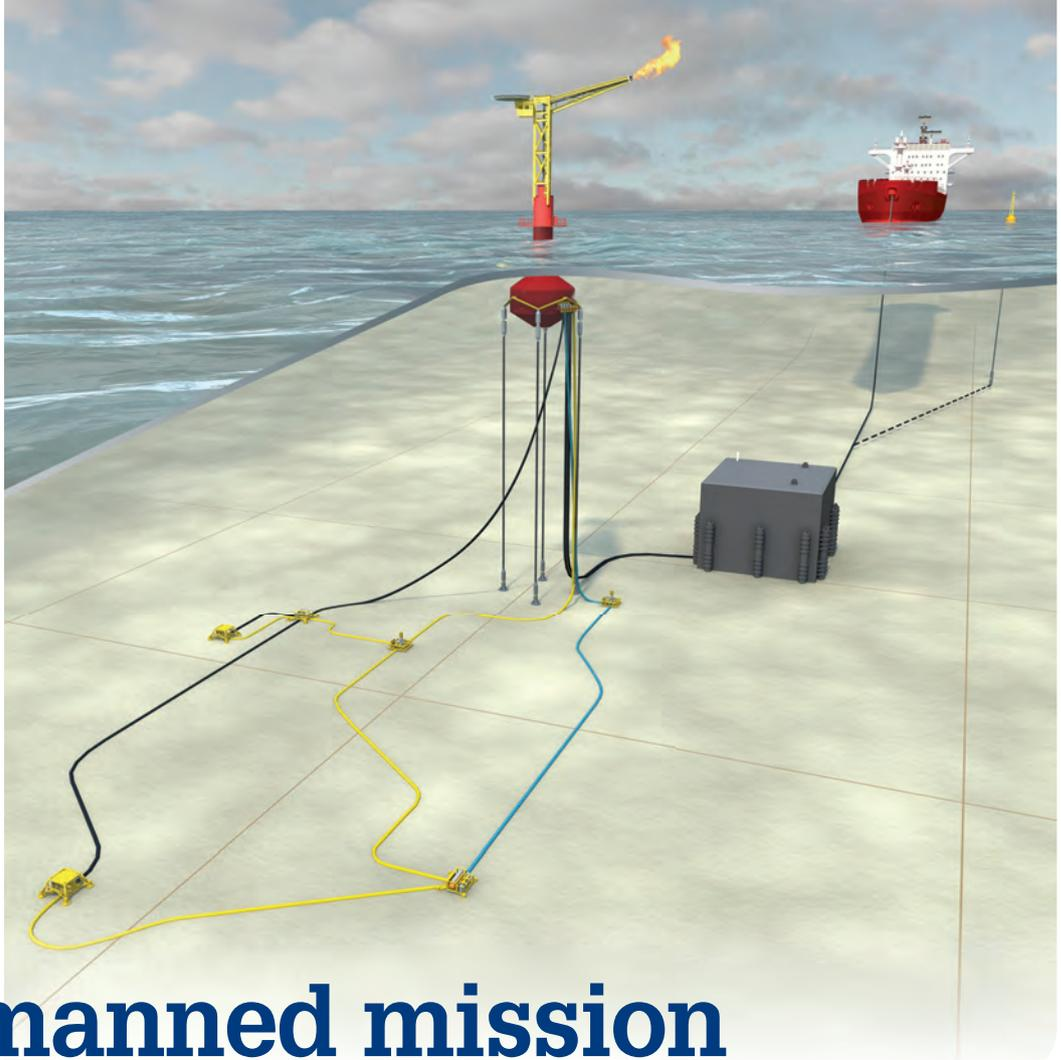
**ABT Oil & Gas' production buoy concept.** Image from ABT Oil & Gas.
