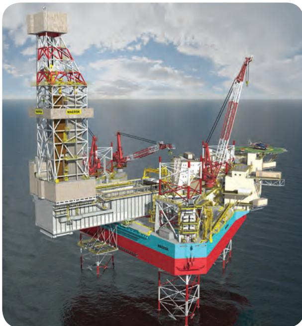
Another jackup under construction at the Jurong yard is the Category J Noble CJ-70—based on the GustoMSC CJ70. The unit is due 1Q 2016 and will undergo acceptance testing in the UK, according to Noble's latest fleet status report. It can operate in up to 492ft water depth, and drill to 32,000ft. It has a variable deck load of 17,600kips, with quarters for 150. Noble's CJ-70 will work Statoil's Mariner field in the UK North Sea, approximately 150mi. east of the Shetland Islands.
