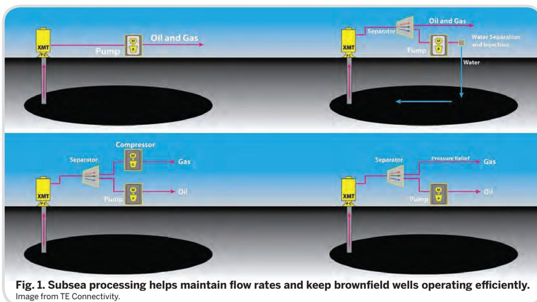
**Fig. 1. Subsea processing helps maintain flow rates and keep brownfield wells operating efficiently.**
