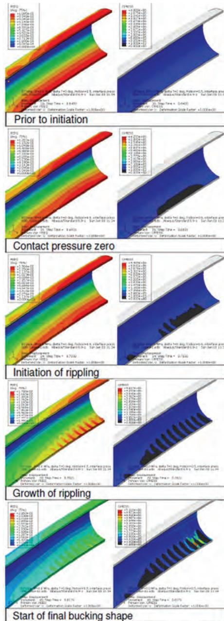
**Image 1: FEA analysis of pipe response to stress.** The diagram at the top shows the pipe at rest. As bending force is gradually applied, ripples begin to grow in the CRA liner. At the bottom, the pipe is beginning to buckle. Image from INTECSEA
