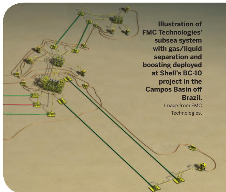
**Illustration of FMC Technologies' subsea system with gas/liquid separation and boosting deployed at Shell's BC-10 project in the Campos Basin off Brazil.**
