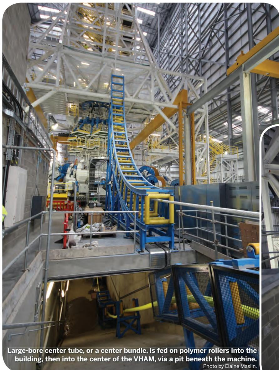
Large-bore center tube, or a center bundle, is fed on polymer rollers into the building, then into the center of the VHAM, via a pit beneath the machine.
