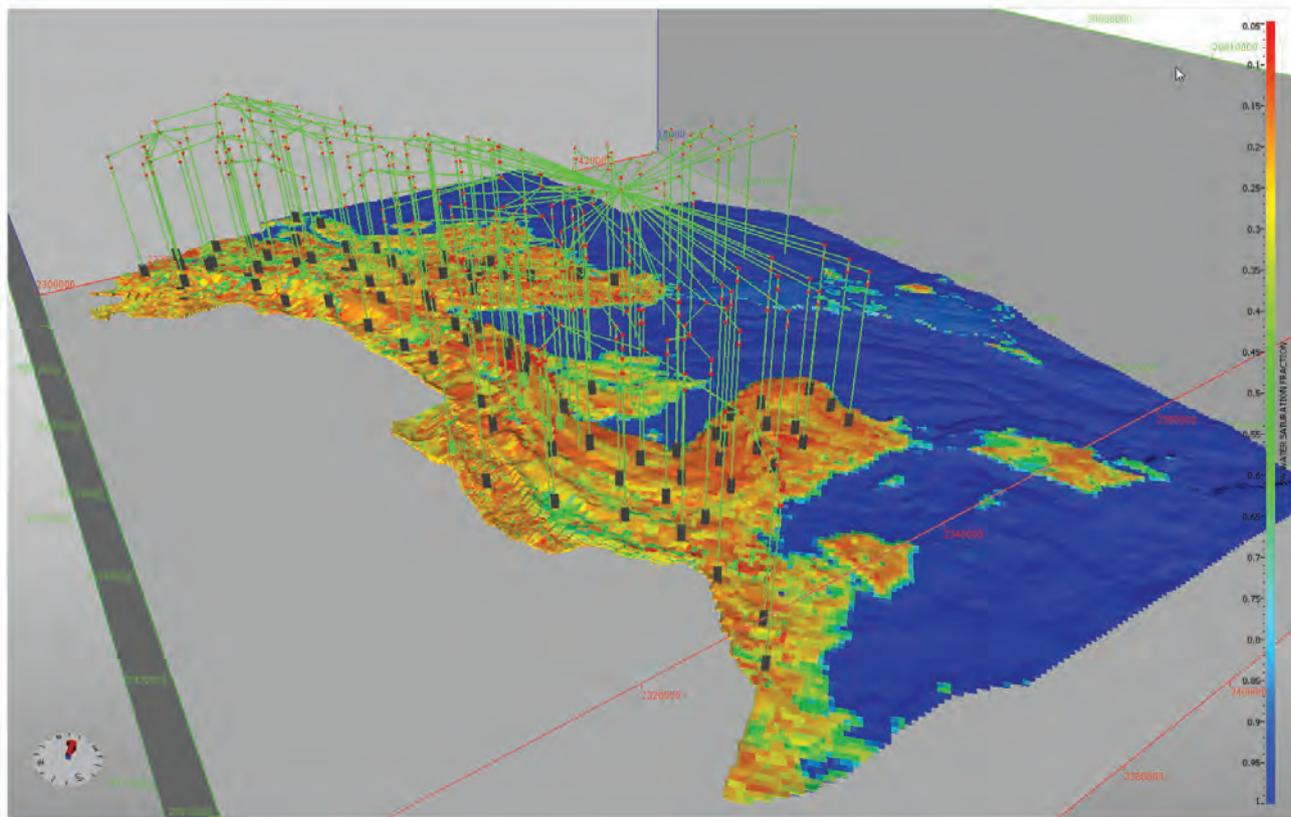
**Subsurface and well planning reservoir simulation model for Prosperidade field offshore of Mozambique.** Image: Anadarko.
