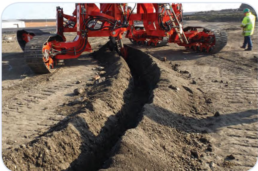
Hi-Traq's steering capabilities improves the minimum trenching radius.
