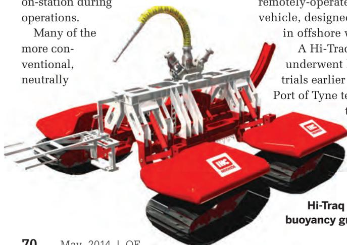
**Hi-Traq streamlined chassis with buoyancy grabs and tooling cylinder.**
