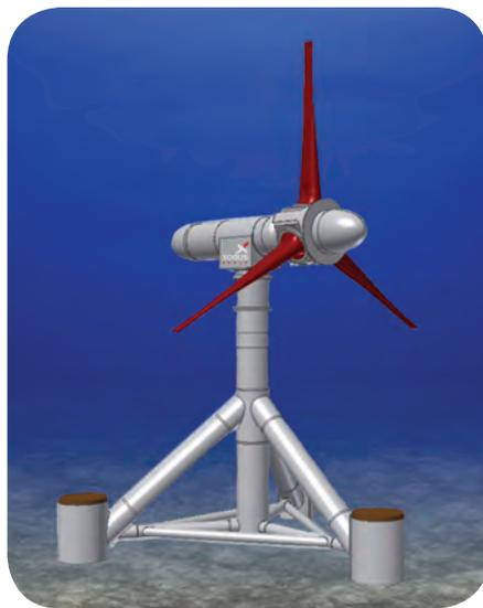
**Fig3 – Typical Horizontal Axis Tidal Turbine (HATT)**
