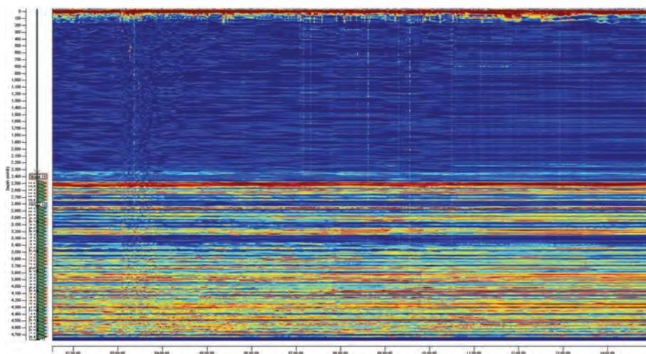
Time verse Depth waterfall showing DAS recording of in-flow at the production zone of a horizontal well.
