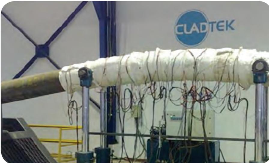
**Image 4: CRA-lined pipe wrapped in insulating material. This test demonstrates a pressurized and heated pipe placed under a 1.5% strain load.**
