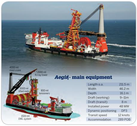
plus lifted reels and the use of a pipelay abandon or recover system for deepwater lowering. The pipelay tower is called an R J tower by HMC, because it can perform reel-lay and J-lay, by using different ways to hold the pipe – friction clamps and hang off collars.
