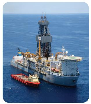
Pacific Drilling's *Pacific Santa Ana* drillship, classed by ABS, has been outfitted with dual gradient drilling technology for Chevron's operations in the Gulf of Mexico. Photo from Pacific Drilling.
