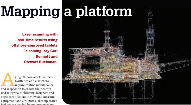
Linking together data from multiple surveys to create whole platform virtual model Images from Wood Group ODL.
