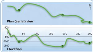
Possible pipeline route with tie-in points for subsea pressure boosting.
