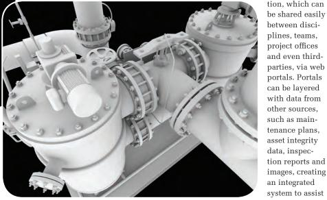
A 3D visualization developed from scan data.
