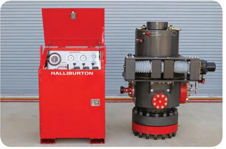
RCD5000 Big Bore with the hydraulic clamping device standing beside a hydraulic closing unit. Photo from Halliburton.
