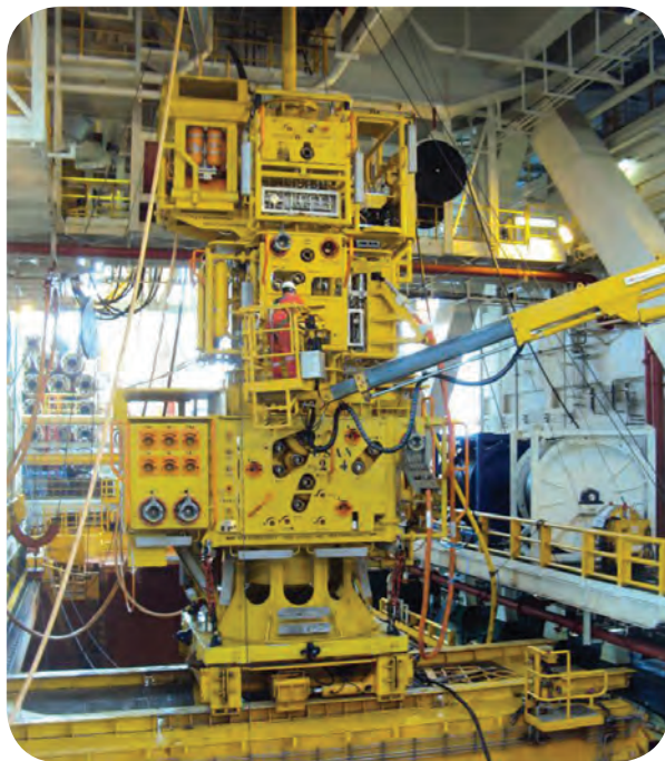
An emergency disconnect package and lower riser package. Image from OneSubsea.
