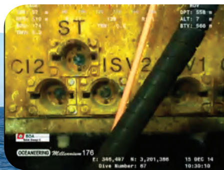
Left: Tree ROV panel. Right: The insert safety valve ROV bucket. Photo from Stone Energy.
