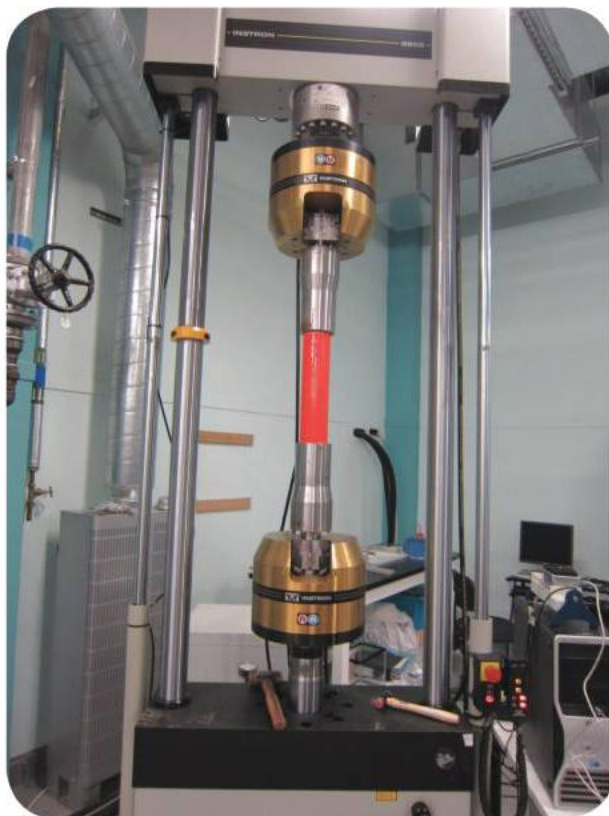
Interventor characterization testing at University of Strathclyde. Photo from Hydrasun.
