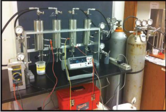
High-pressure high-temperature testing facilities with resistance measurements. Image from Dr. C. Vipulanandan.
