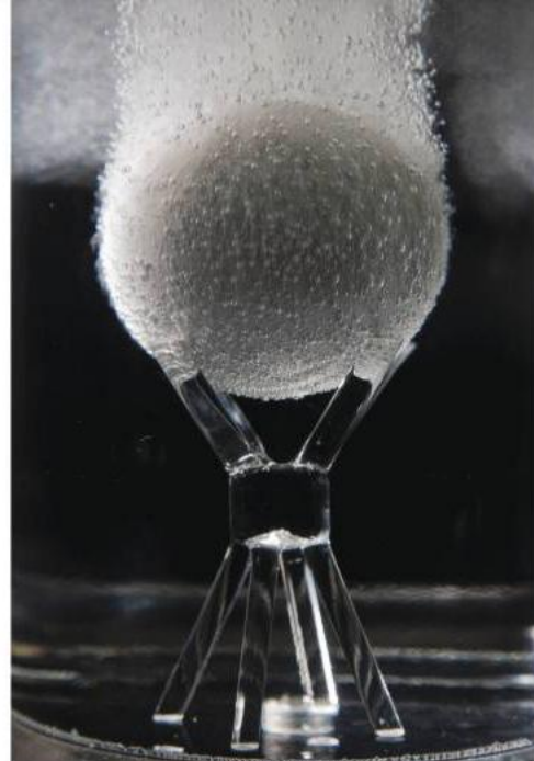
The IN-Tallic frac ball, also made from CEM nano-engineered material, that illustrates how this material completely disintegrates in wellbore fluids.
