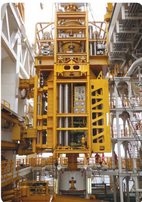
s the industry moves closer to the deployment date for the first blowout preventers (BOPs) rated to withstand pressures of 20,000psi (20K), there is a notion that these new BOPs are "the same thing, just bigger." While technically correct, this vastly underestimates the true impact of this new technology on the entire drilling system. Ensuring successful drilling campaigns with 20K well control systems requires a new approach to specification, acquisition, operation and maintenance procedures.
