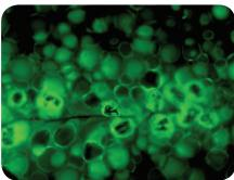
"Smart beads," filled with chemicals that can fill cracks caused by pipeline corrosion, are added to a coating that is painted on the asset before it is deployed. Terahertz spectroscopy devices enable maintenance personnel to identify where the beads have burst and the pipe requires repairs. Images from Battelle.
