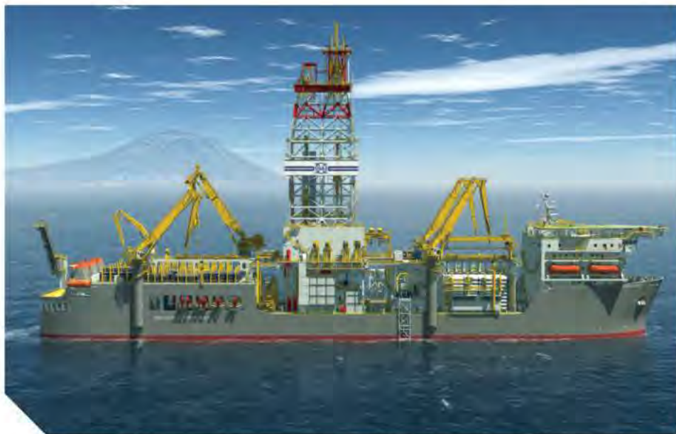
Friede & Goldman's DS3810 deepwater drillship design, which is being evaluated by ABS for AIP, is designed to drill in 14,750ft (4500m) water depth. Image from Friede & Goldman.
