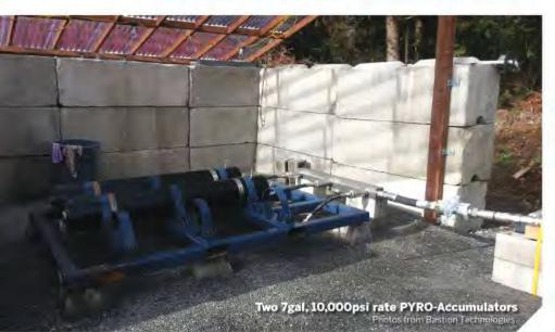
as charged accumulators are widely used as the hydraulic power source for subsea blowout preventers (BOPs). To compliment these conventional accumulators, Bastion Technologies has developed a PYRO-Accumulator, which uses a solid fuel source, like the booster rockets used to send vehicles into space, instead of gas.
