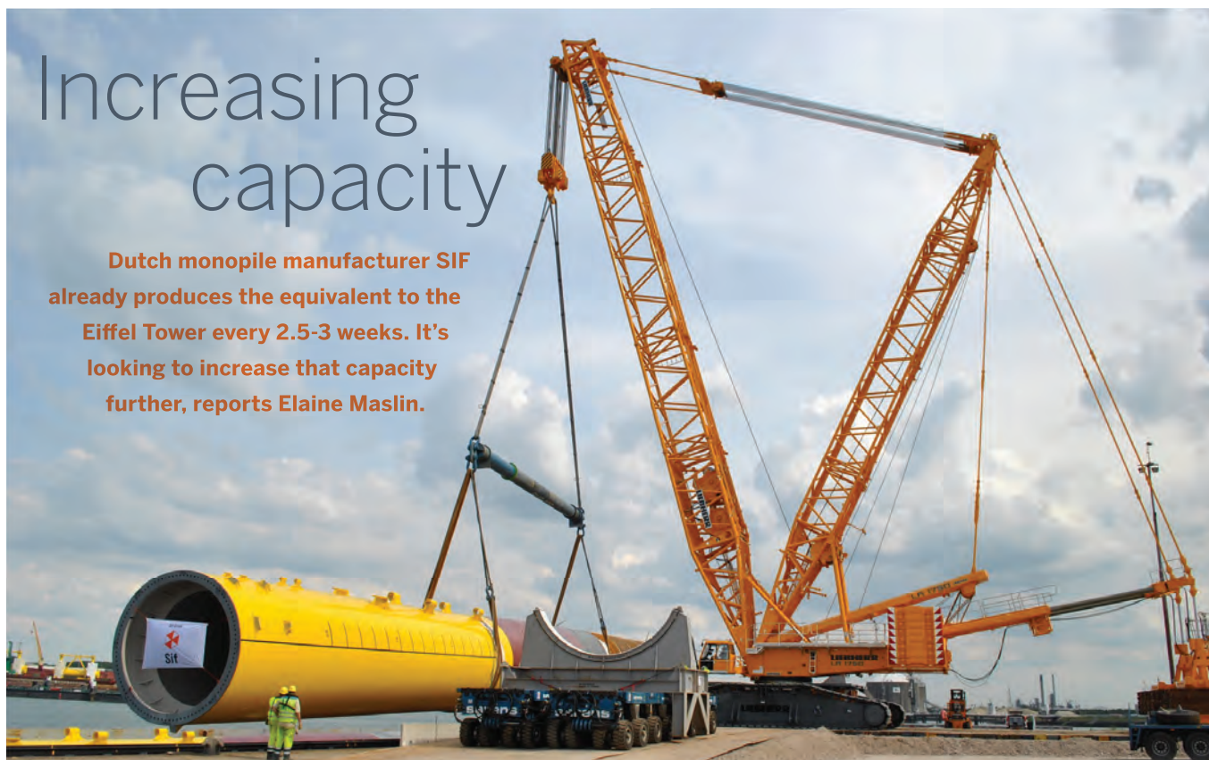
SIF monopile offloading. Images from SIF.
