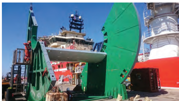
Assembly of a Rental Reel at Customers Shore Base
