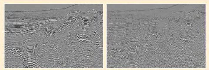
The reprocessed multiclient 2D line survey (left) and the original shot in 2001 (right) Images from TGS.
