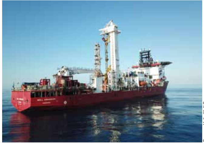
Helix Well Ops' Well Enhancer light well intervention vessel, used on the McCulloch subsea P&A campaign.
