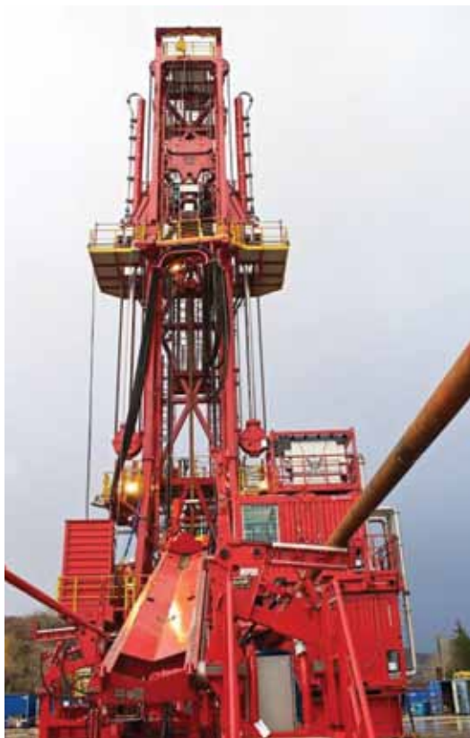
Halliburton's modular rig , for the Jotun B P&A operations.
