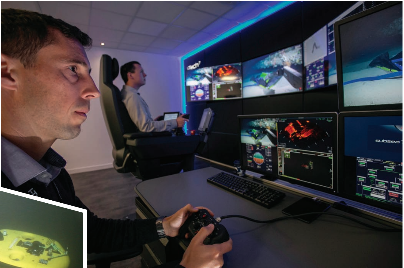
Remote operations are also being done with ROVs. This is i-Tech 7's onshore control center for ROV operations.
