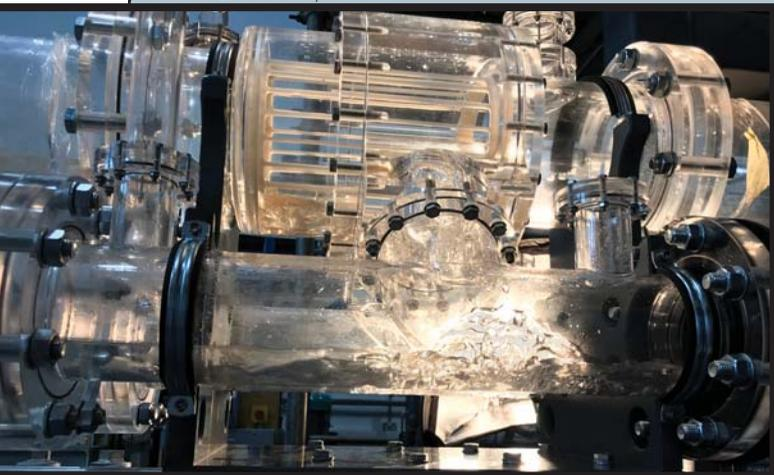
**PDG Unit in Testing:** A scale model test of the pseudo dry gas system has been put through its paces.
