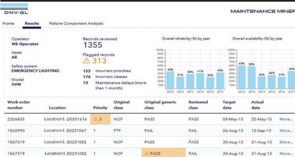
Figure 1: Web tool developed by DNV GL to review free-text maintenance records using ML
