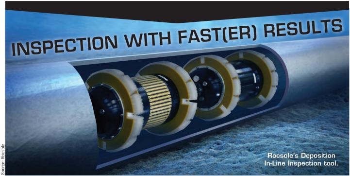
Finland's Rocsole is hoping to provide operators with better, faster insight into their pipelines through a new compact inline sensor and a large dose of data analytics. Its inspection tool uses electrical tomography and digital signal processing to measure conductivity and permeability values within a pipeline. These are then analyzed to determine the content – fluid and solid – of pipelines or vessels, such as separators.
