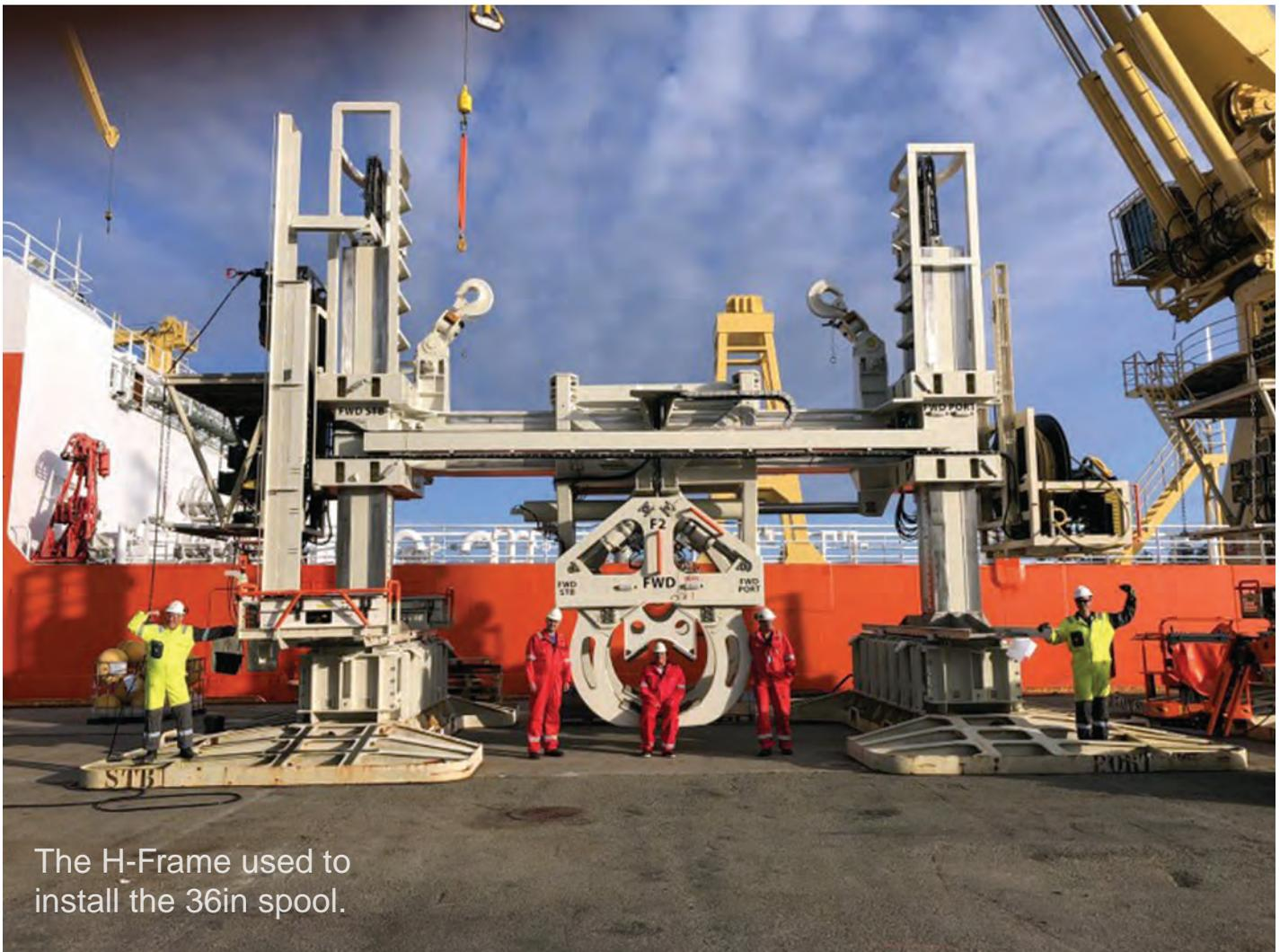
The H-Frame used to install the 36in spool.
