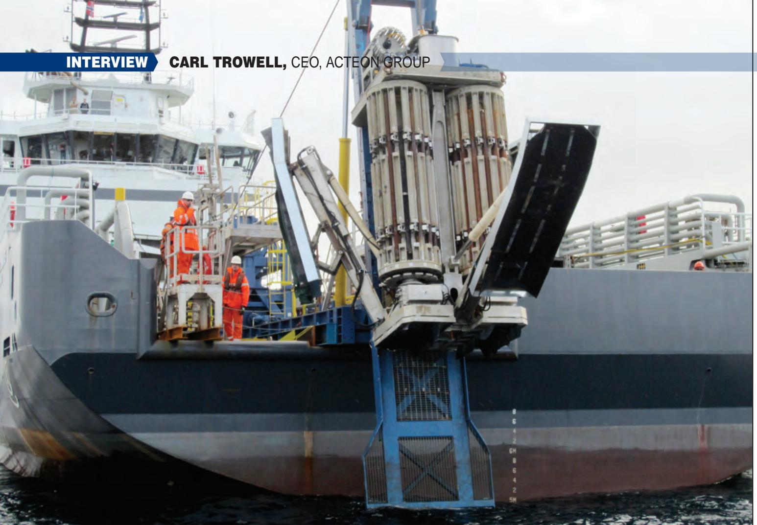
farms where the foundations are getting more complicated. Rock soil parameters are important, and to give you one example, we've developed a new remotely operated sea floor drill specifically for shallow water, unconsolidated sands relevant to the renewables market. We've been doing this for years in the deep water for oil and gas, but we've particularly developed a new product for the renewables market.
