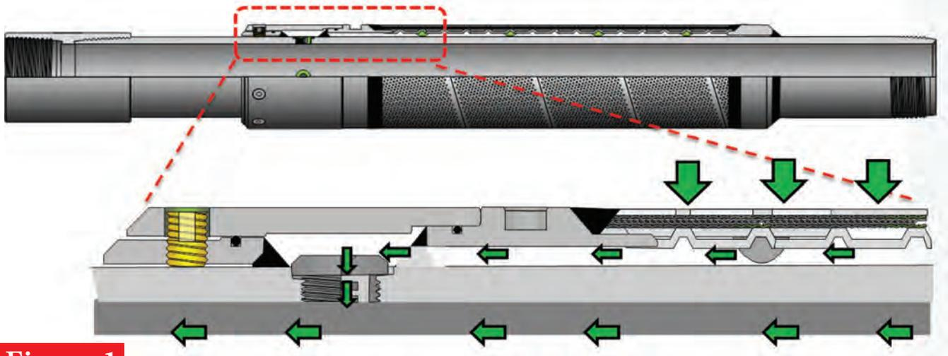
**Figure 1** AICD unit mounted into sand screen joints illustrating production flow path.
