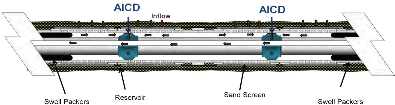
**Figure 2** Retrofit AICD completion in existing standalone screen with the production flow path.
