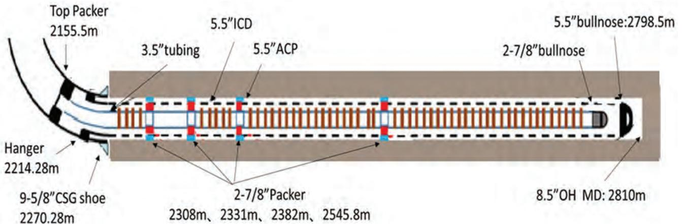
**Figure 3** The retrofitted AICD completion schematics.
