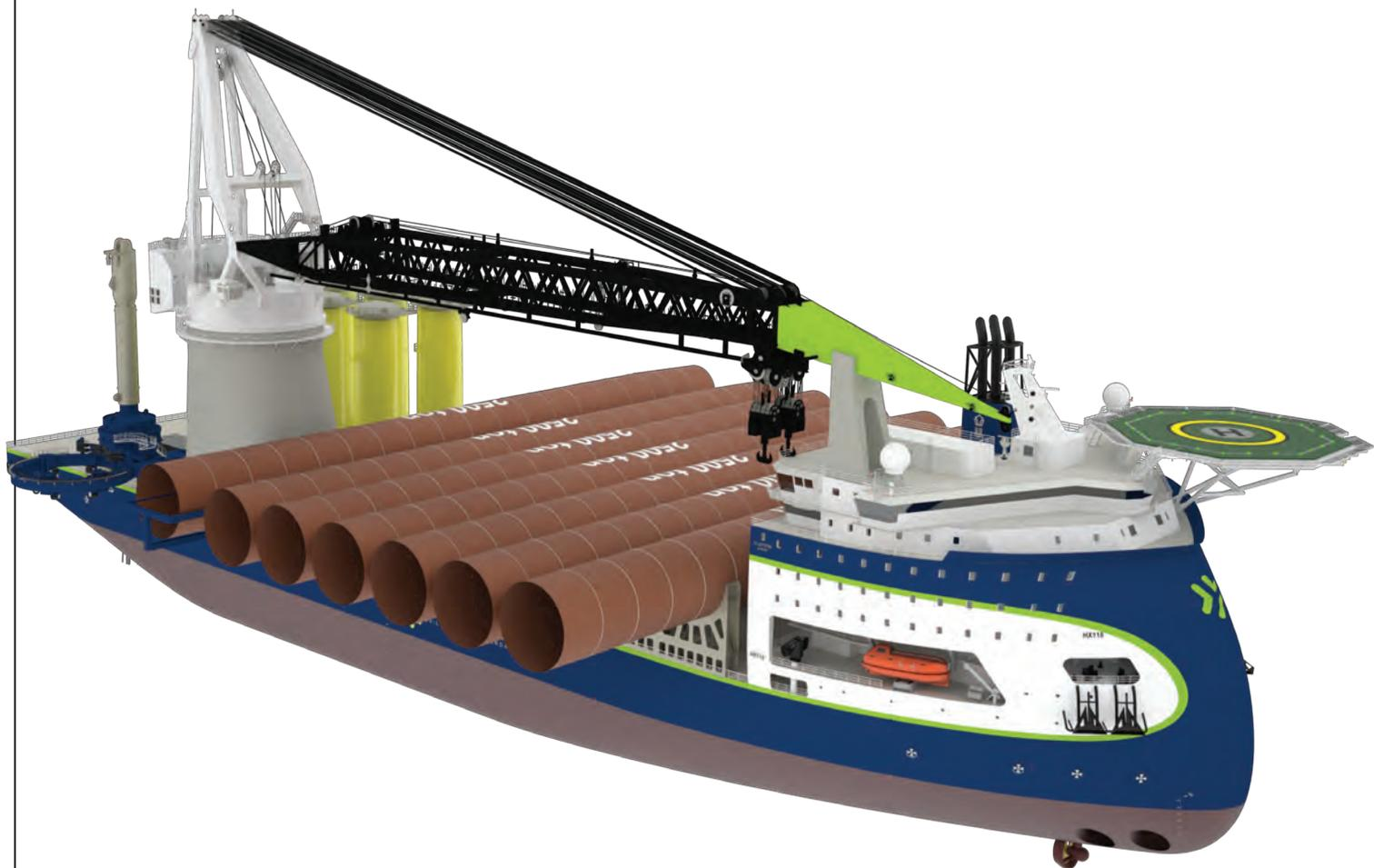
bines. The ship-shaped dynamically positioned vessel will be about 230 meters long by about 60 meters wide, with accommodations for 160 people on board and equipped with a 6,000-ton Huisman crane.
