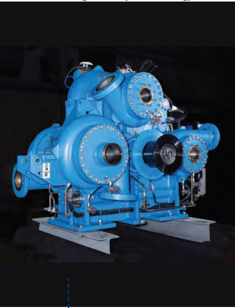
MAN Energy Solutions provide multi-stage compressors for CCS applications.
