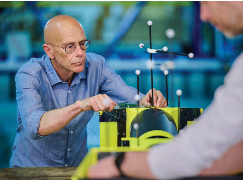
THE FRONT OF THE MACHINE HAS THIS BIG SLOPE PLATE THAT ENSURES THAT THE BOW ALWAYS STAYS SUBMERGED. WAVES ARE OVER TOPPING (THE UNIT) AND THAT'S A NATURAL LOAD SHEDDING MECHANISM.
