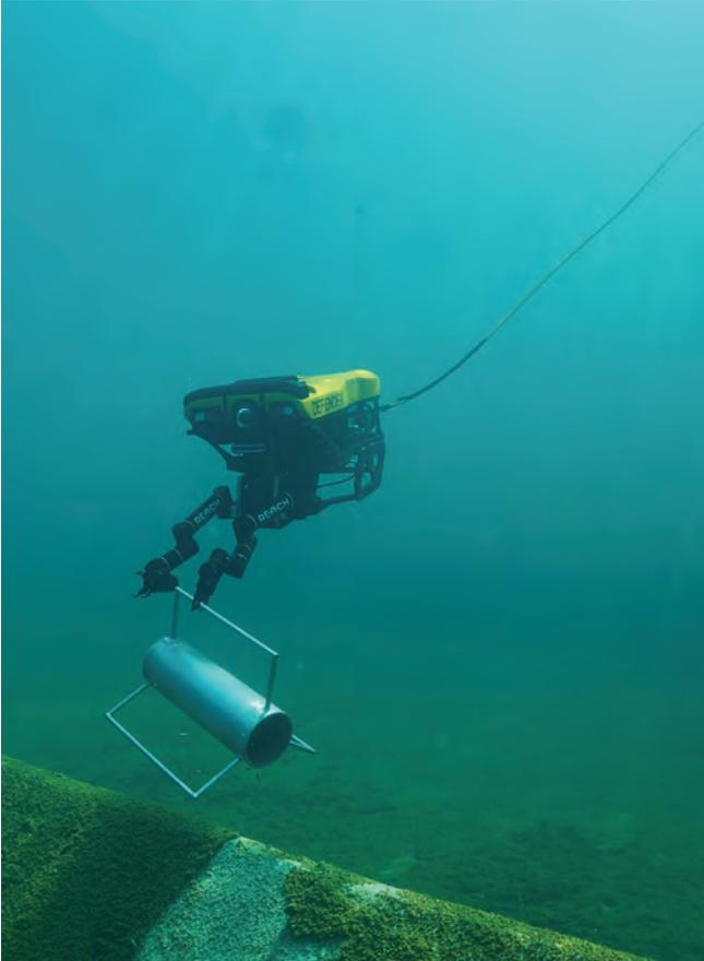
**REACH ROBOTICS HAS RELEASED ITS NEW X7 SUBSEA MANIPULATORS WHICH ENABLE OPERATORS TO EXECUTE DEXTEROUS INTERVENTION OPERATIONS THAT TRADITIONALLY HAVE BEEN PERFORMED BY EITHER DIVERS OR WORK CLASS ROVS.**
